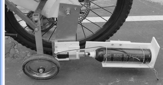
Modified aircraft landing gear mechanism by a linear actuator (489 N peak force, 2-inch stroke) for wheel retraction.
